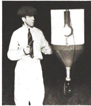
Last year in New Jersey, the heart of the beetle plague, the Type G-5 ultra-violet lamps trapped more beetles in an hour than any other method.
